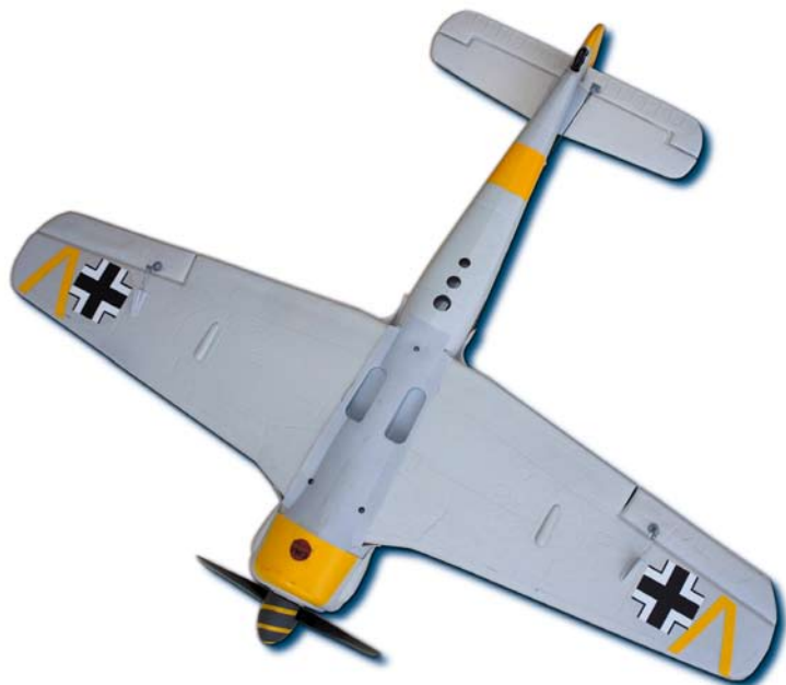
Above: Underside reveals the finger grip for hand-launching and air cooling outlets
