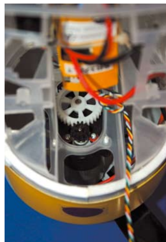
Above: 480-motor and gear-train face rearwards
