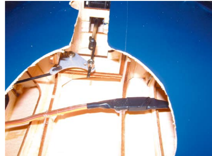
Above: Retract operating bell crank and rods are pre-installed
