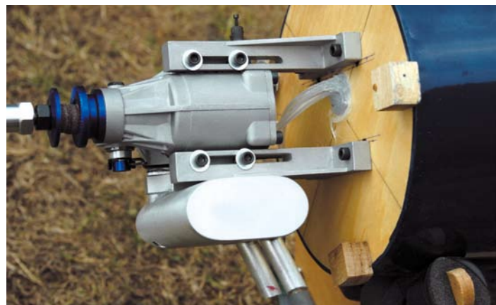
Above: The adjustable slots in the T-mount makes installation a doddle
