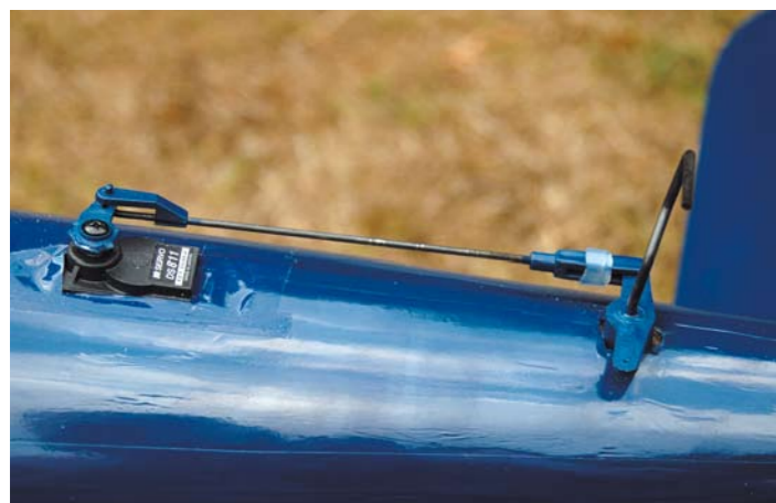
Above: Tailwheel steering and rudder servo installation
